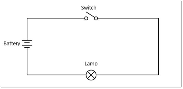
This circuit would work; however, in order for the bulb to be lit the switch would have to be closed.
